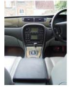
2. Start by removing the cup holder, one of the screws for the centre console is hidden under here:
