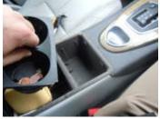
3. Remove the screw under the cup holder and the one located in the main compartment at the back left.
