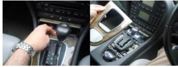
6. Start to pull the main surround away. This just unclips from several locatons. A couple at the top, a couple on the sides and a couple near to the park brake lever.
