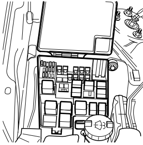
FRONT POWER DISTRIBUTION FUSE BOX
