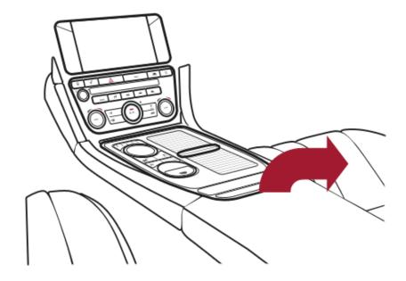
2.2 Insert the USB stick containing the downloaded map data into the slot.
