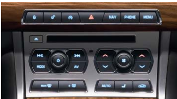
Center stack switches
