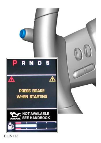
Scroll through the trip menu to access the engine oil level display.
