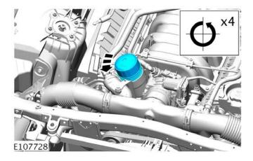
Loosen the element cover 4 complete turns to allow engine oil to drain from the filter cover. Make sure that the O-ring seal is exposed.
