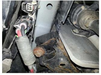
8. Remove cooling fan retaining bolt (1) and clip (1) on passenger side of the assembly
