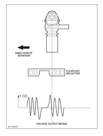
The reluctor is manufactured to have a 'tooth' pattern based on 60-2 pattern, where there are 58 teeth in total at  $6^{\circ}$  intervals. The two teeth are removed to provide a hardware reference mark, with a centerline that is  $21^{\circ}$  BTDC on cylinder 1, RH bank.
