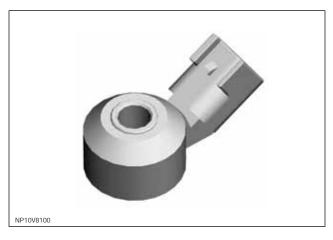
Each sensor monitors engine knock by converting the engine block noise into a suitable electrical signal, which is then transmitted back to the ECM via a twisted-pair cable. The signal is processed within the ECM to identify the data that characterizes knocking.
