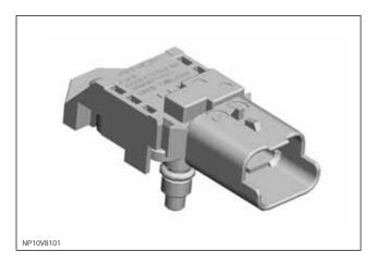
The MAP sensor is mounted on the top of the engine, at the front behind the throttle body. The purpose of the sensor is to measure the absolute pressure in the intake manifold and provide information to the ECM, which will determine the injection time.
