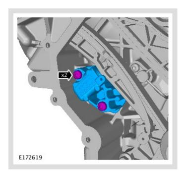
Remove the timing chain tensioner.
