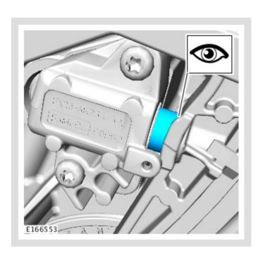
The piston should apply tension to the timing chain guide.
