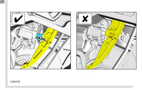
The timing chain tensioner must maintain tension on the chain guide. If the piston can be pushed back so the chain guide contacts with the body of the tensioner, the tensioner is not correct. Repeat steps 87-93.
