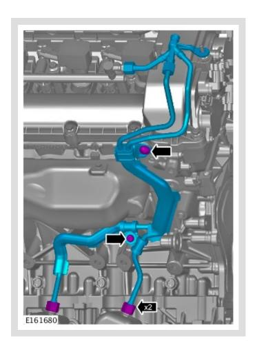
Remove and discard the high-pressure fuel supply lines.
