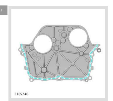
Apply RTV sealant (Loctite 5901G) to the areas shown, install the component, and tighten the bolts within 7 minutes.
