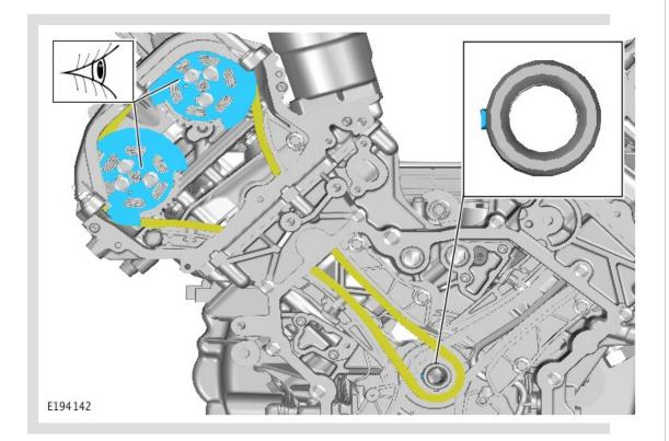
Check that the position of the Variable Valve Timing (VVT) unit and crankshaft keyway are positioned as indicated. If the VVT units are not positioned as indicated, rotate the crankshaft clockwise until the correct crankshaft keyway and VVT unit positions are achieved.
