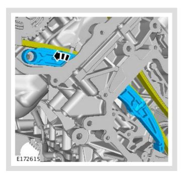
Install the timing chain guide.
