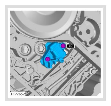
Remove the timing chain tensioner.
