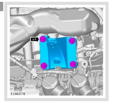
Remove the right engine mounting bracket.
