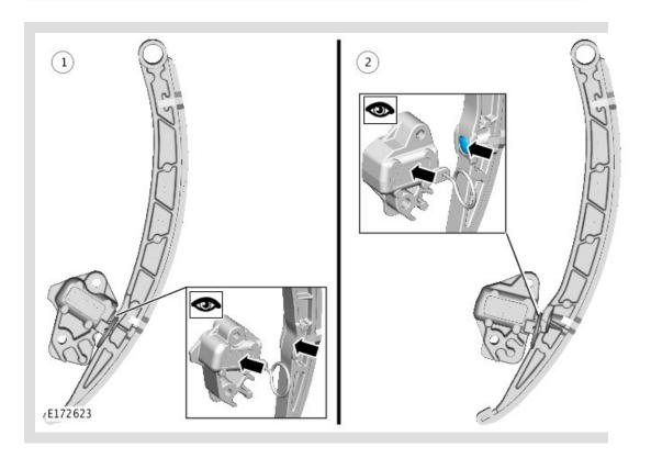
Using the illustration, identify which timing chain tensioner and guide is currently fitted to the vehicle. Make sure the vehicle is assembled using components shown in section (2) of the illustration only.
