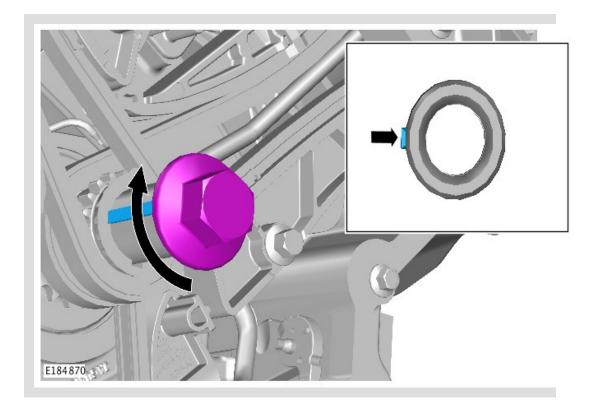
Rotate the crankshaft clockwise 90 degrees until the crankshaft keyway is positioned as indicated in the illustration.
