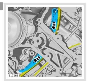
Remove the timing chain guide.
