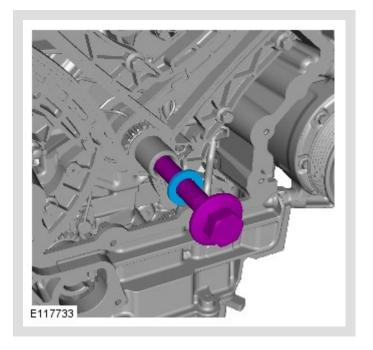
Install the crankshaft pulley bolt.
