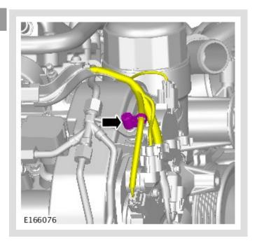
This fuel pipe can be re-used, inspect for signs of damage. Renew if necessary.
