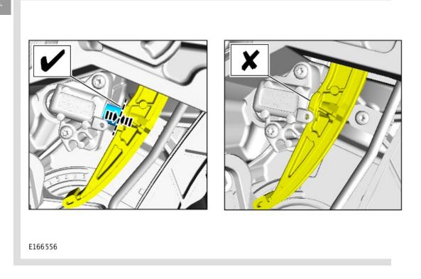
The timing chain tensioner must maintain tension on the chain guide. If the piston can be pushed back so the chain guide
