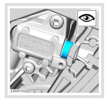
The piston should apply tension to the timing chain guide.
