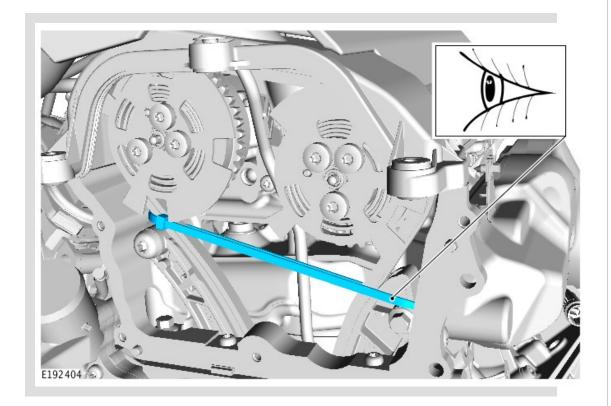
Loosely install the tie strap around the timing chain guide on the non-tensioned side and the timing chain on the tensioned side, as illustrated.
