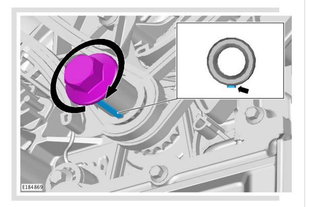
Rotate the crankshaft clockwise until the crankshaft keyway is positioned as indicated in the illustration.
