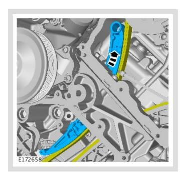
Install the timing chain guide.
