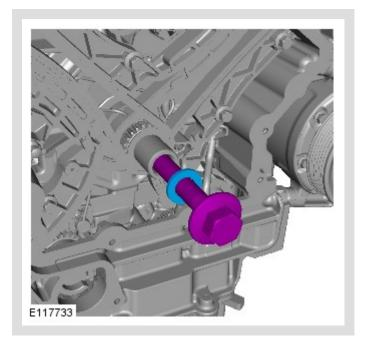
Remove the crankshaft pulley bolt.
