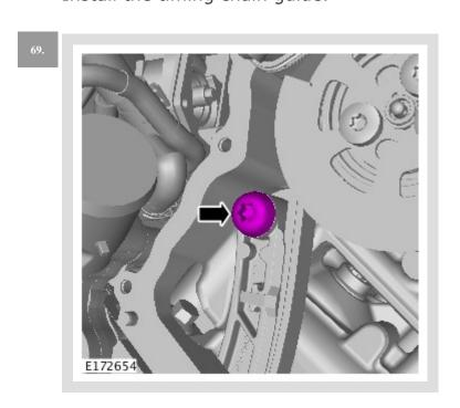
Install the timing chain guide bolt.
