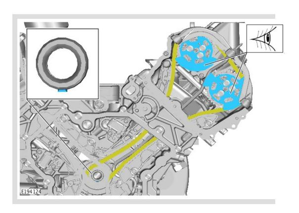
Check that the position of the Variable Valve Timing (VVT) unit and crankshaft keyway are positioned as indicated. If the VVT units are not positioned as indicated, rotate the crankshaft clockwise until the correct crankshaft keyway and VVT unit positions are achieved.
