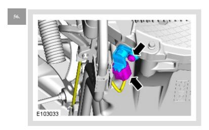
Remove the crankshaft position sensor.
