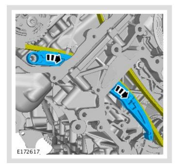
Remove the timing chain guide.
