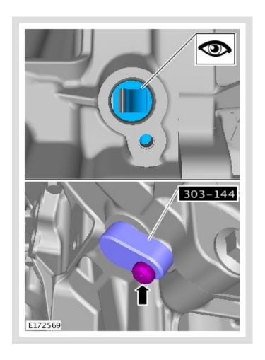
Install the crankshaft timing tool, if required rotate the engine to the correct position.
