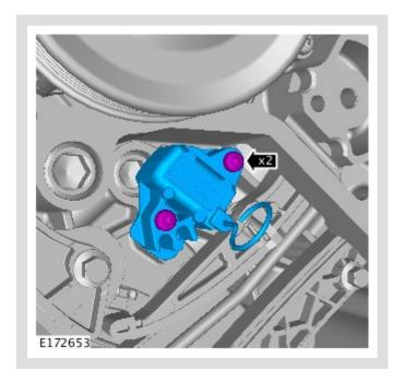
Install the timing chain tensioner.
