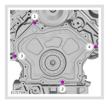
Tighten the lower timing cover bolts within 7 minutes.
