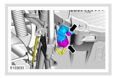
Install the crankshaft position sensor.
