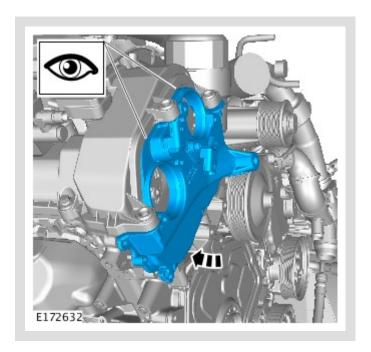
Tighten the retaining bolts in the indicated sequence.
