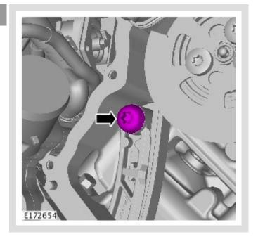
Remove the timing chain guide bolt.
