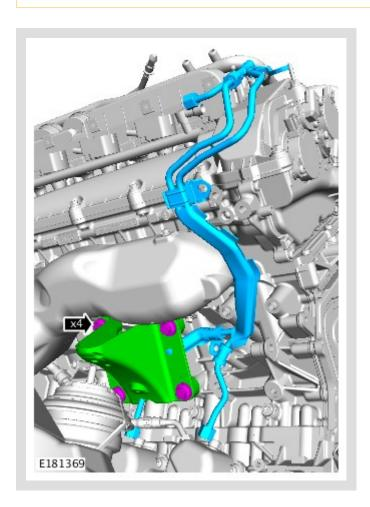
Install new high-pressure fuel supply lines. Loosely position the high pressure fuel pipes but do not tighten the unions at this stage.
