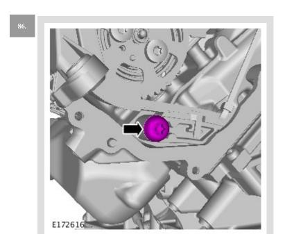
Install the timing chain guide bolt.
