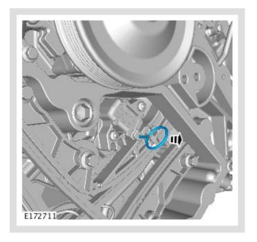
Release the retaining pin.
