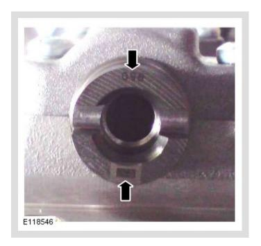
Carefully rotate the camshafts if the position is not as shown.
