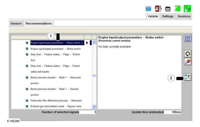
11. Select 'Engine input/output parameter - Brake switch' (1) then click on the icon shown (2).
