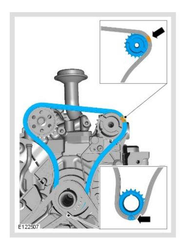
Install the lower timing chain making sure the coloured chain links align correctly with the fuel rail high-pressure fuel pumps camshaft and crankshaft sprocket markings.
