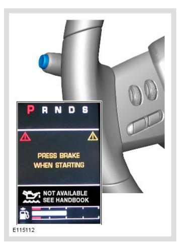
Scroll through the trip menu to access the engine oil level display.
