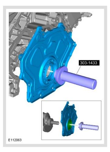
Install the bolts, but do not tighten fully at this stage. *Special Tool(s):* 303-1433
