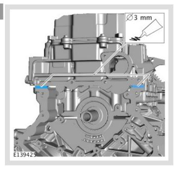
Apply RTV sealant WSE-M4G323-A6 (Loctite 5901G) to the areas shown, and tighten the bolts within 7 minutes.
