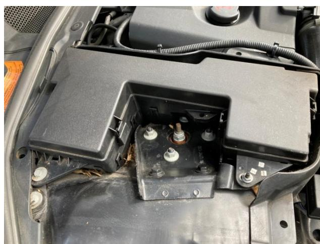
There are four clips holding this on. These just have to be 'squeezed' to get the cover off. Once off. The fuses and relays are revealed.
