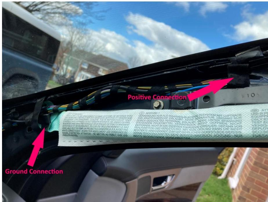
The positive connection is tucked behind the metal bracket you can see. It should be eased out for access. Care should be taken doing this to ensure the ribbon cable is not damaged.
