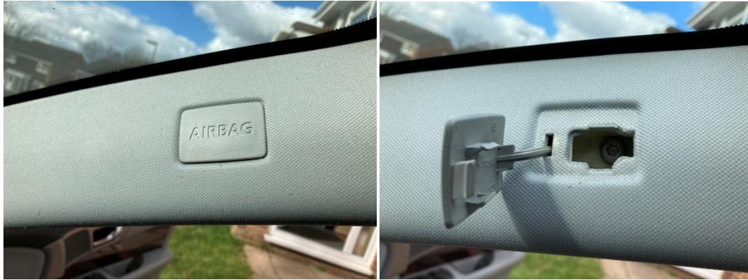
This will reveal a T30 Torx bolt which will need removing.
