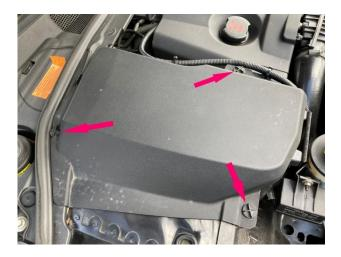
Watch out for these. They can easily go 'ping' into the bowels of the engine bay as you pull the cover off
