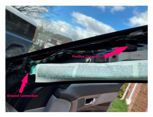
The positive connection is tucked behind the metal bracket you can see. It should be eased out for access. Care should be taken doing this to ensure the ribbon cable is not damaged.
