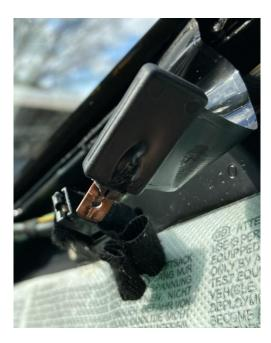
Cleaning the connector proved a 100% cure to my faulty heated screen.
