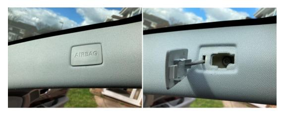
This will reveal a T30 Torx bolt which will need removing.
