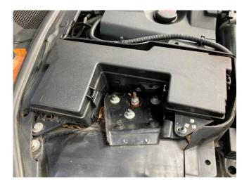
There are four clips holding this on. These just have to be 'squeezed' to get the cover off. Once off. The fuses and relays are revealed. I have indicated the items of interest.
