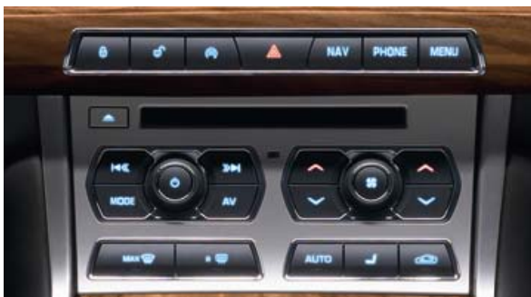
Center stack switches
