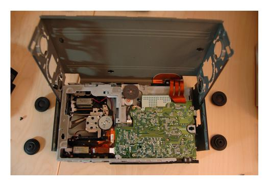
Now, the actual repair/adjustment. On the lower left hand side of the picture below, you will see this worm/wheel drive gear. There was a small gap between them, causing the worm to not driving the gear, and therefore, failed to pick up the CD.
