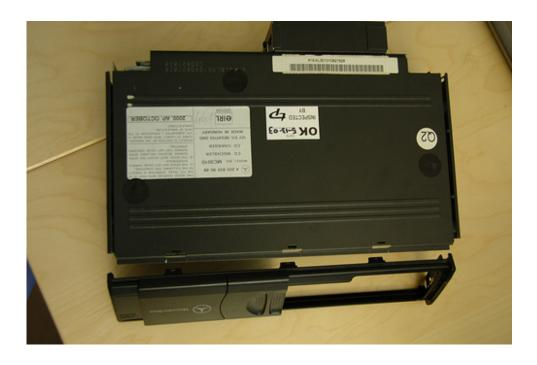
Then, remove the springs that suspends the internal casing for anti-vibration using a long nose plier.
