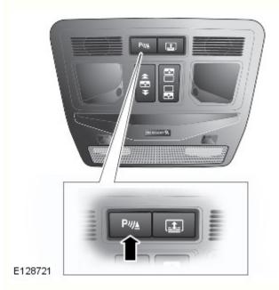
The parking aid switch is located in the instrument panel switch pack, above the touch screen. The switch is the LH switch with an integral LED .
