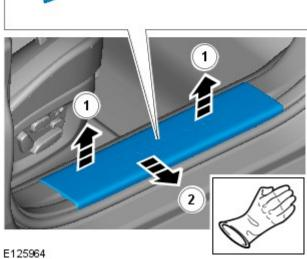
CAUTION: Make sure that the component is correctly located on the locating dowels.
