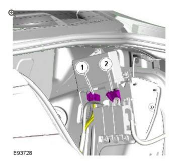
Connect the electrical connectors in the sequence shown.
