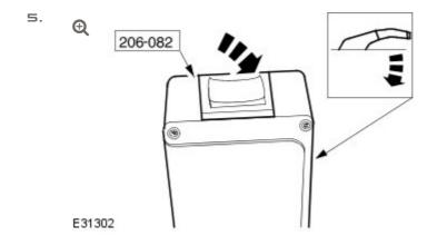
Release the parking brake cable tension.
