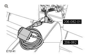
Connect the special tool to the parking brake module.
