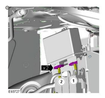
Disconnect the 2 electrical connectors from the parking brake module, in the sequence illustrated.
