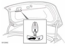
The release handle glows in the dark and is located on the inside of the luggage compartment lid. To open the luggage compartment from the inside, pull the handle while pushing the luggage compartment lid upwards.
