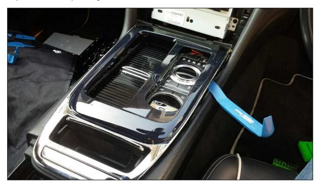
You can then lift out the trim and unplug the electric cables at the back to free the trim.
