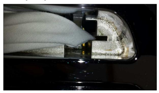
Here is the button with the flat spring and the 2 rubber stoppers. The 2 areas highlighted need to be cleaned of grease.
