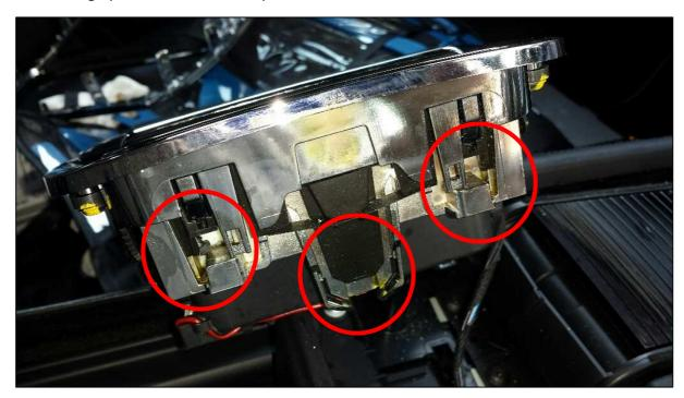
To get the button out of the trim you need to use a flat screw driver to lift the tabs gently either side and then push the button out. There are 2 rubber stoppers that fall out easily as well as the flat spring.
