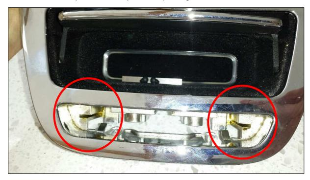
Using the white spirit and a paintbrush I cleaned out the grease. I also wrapped a cloth around a flat screwdriver to get into the groove.
