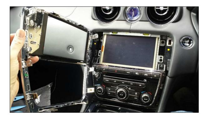
You then need to unscrew the trim below the screen. There are 4 screws to loosen at each corner.
