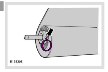
Remove the retaining clip.
