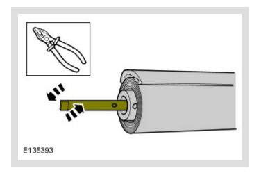
Using a suitable tool, rotate the shaft 10 full rotations counter clockwise.
