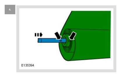
Align the holes between the shaft and the blind.
