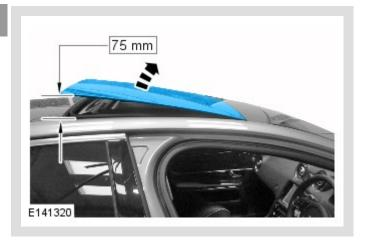
Open the roof opening panel glass to the full tilt position.
