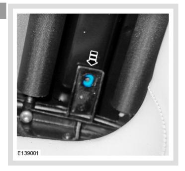
Slide the washer in from the centre of the vehicle until it is aligned with the threaded hole.
