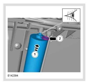
Remove the retaining clip.
