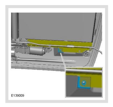
If not already installed, install an adhesive pad above the front fixing hole.
