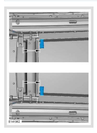
Slide the blind foot along the guide until it is level with the foot on the other side of the vehicle.
