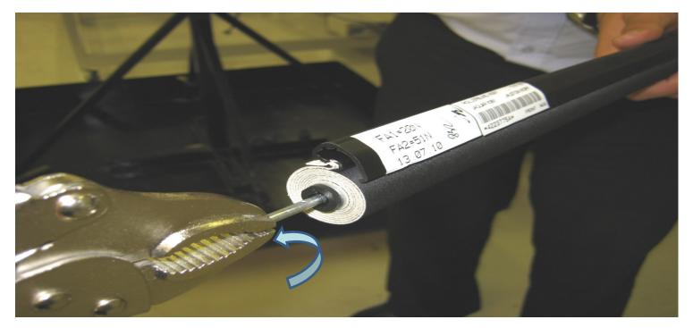
With blind in unwound state, hold in orientation shown, grip flat of metal shaft tightly in clocking pliers. Hold blind in position and rotate locking pliers **anticlockwise** to increase tension.
