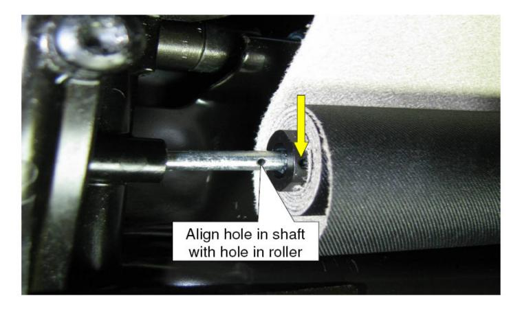
Note the location of the hole in the shaft and line up the hole in the roller to it for pinning.
