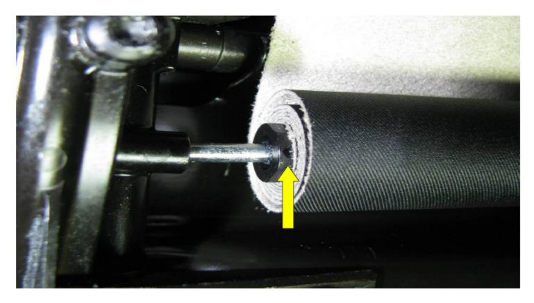
Once lined up insert a pin into the hole to lock the blind in place. Note: Use the correct blind pin, but if unavailable use a hardened pin like an Allen key or drill bit, the diameter of the pin is approx 1mm.
