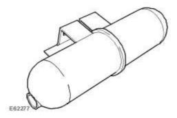
The AIR vacuum reservoir is located on the right-hand side of the engine bay.
