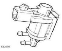
The ECM switches on the AIR switching valve with a one second delay after initiating AIR pump operation. When the AIR switching valve is open, a steady vacuum supply is allowed through to open the vacuum operated AIR control valve. When the ECM switches off the AIR switching valve, the valve closes and immediately shuts off the vacuum supply to the AIR control valve. The pump continues to operate for a further five seconds for system diagnostic purposes.
