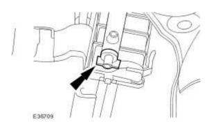
5. Install the radiator splash shield. Radiator Splash Shield (76.22.90)
