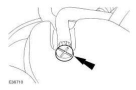
9. Install the coolant expansion tank pressure cap.
