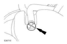
7. Fill the cooling system up to the MAX mark on the coolant expansion tank using a fifty percent mixture of Jaguar Premium Cooling System Fluid or equivalent, meeting Jaguar specification WSS M97B44-D and fifty percent water.
