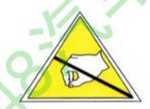
It is displayed near components or assemblies that are sensitive to electrostatic discharge.
