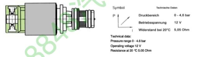
Pressure regulator with falling characteristic (700 mA = 0 bar / 0 mA = 4.6 bar)
