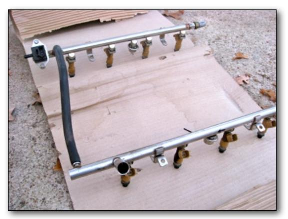
prevent vibration (apparently). As the story goes (I could have some of this wrong), fuel rails on earlier models would tend to vibrate, perhaps due to the high pressure? Jeff (British Auto) referred to something as the "helicopter". I guess the vibration. of earlier models? Anyway, the new fuel rail design was supposed to prevent this (I think). The fuel leak was at the little, upside-down hat between the fuel injectors.
