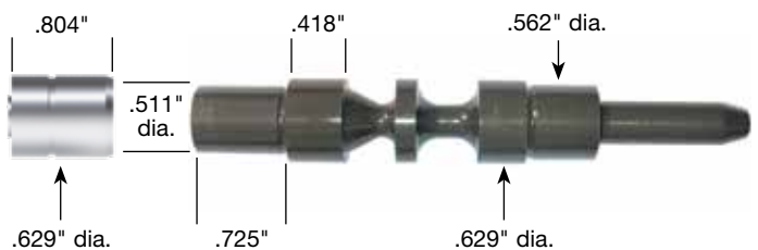
Pressure Regulator Valves and Sleeves Cannot Be Interchanged
