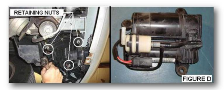
NOTE: TO RELEASE AIR TUBE(S), PRESS DOWN ON THE QUICK RELEASE FITTING COLLAR, WHILE PULLING OUT AIR TUBE(S)
