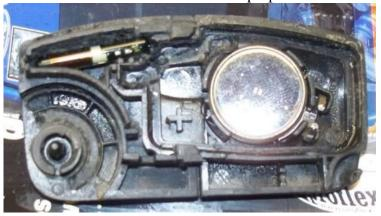
Transponder chip: antenna is the copper looking side and this side is placed to point towards the top of the key Fob. The chip receives power by its proximity to the receiver ring (ignition) & then sends back the code to the car via the chips antenna.
