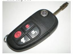
Upper portion of Key Fob with flip out key blade. Notice about 1/8 inch of the transponder showing At the right edge in the middle. It is wrapped in A silicone tube.
