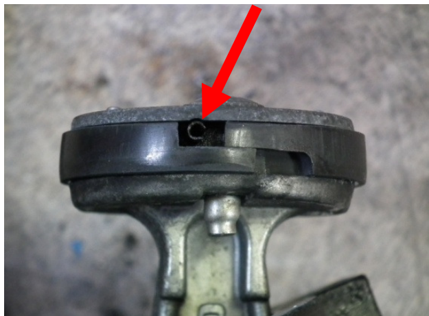
Photo C below, Note old Piston ring fitment, and location pin:
