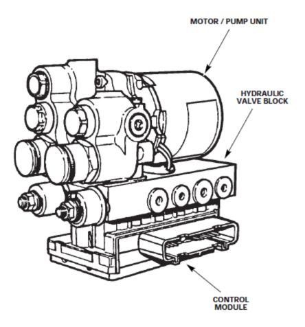
C1095 Pump Motor Resistance Fault Repair Teves Mark IV ABS Module [with or without Traction Control]
