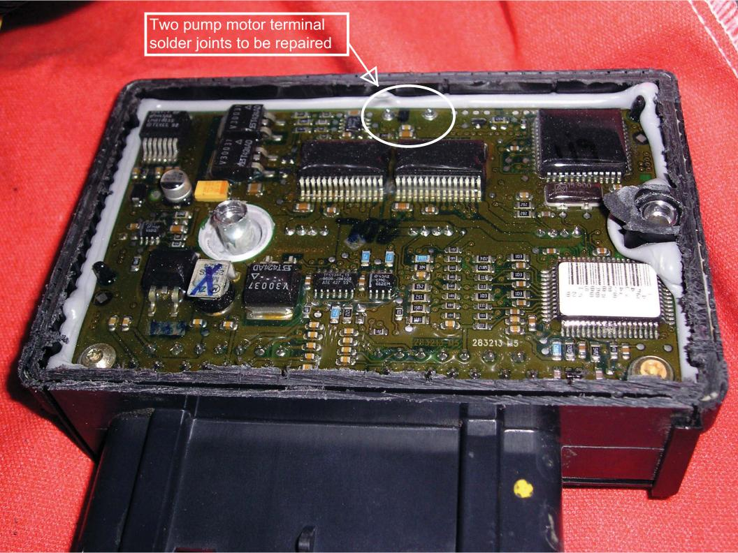
Entire circuit board is layered with an epoxy coating that must be cleared away to expose the two motor terminal solder joints; also, gray RTV at edge must be cut away.
