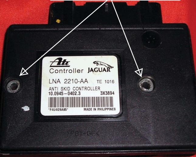
One corner of cover has tab that will be cut through during cutting for removal.
