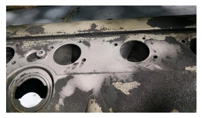
As you can see in the photo below, it did an excellent job at cleaning the inner surface of the well, but it did require you to stop, take off the hood and inspect from time-to-time as you can see an area of unclean surface there. While doing this, the sand is rebounding back into your face (I have a hood with face-shield on, but visibility is still near zero, so it is just "point the nozzle in there, swish it round-and-round a bit, then stop and inspect.
