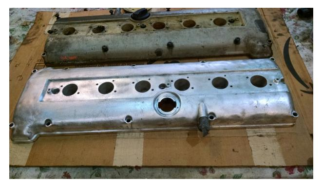
No blasting on the underside. The bright areas you see are where I hit it with a wire brush. As you'll note in later pics, the one below was prior to degreasing.
