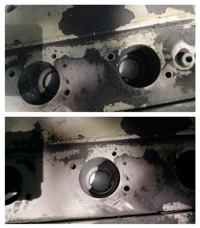
Overall, I just did a quick, spot-blast on this one as "proof-of-concept" or perhaps what the industry I now work in might call "risk-reduction" activity. It assured me that it would get the spark plug wells clean without undue damage to the part, overall.
