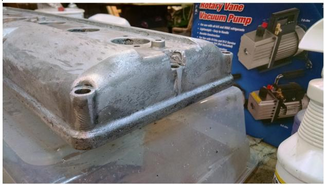
Before proceeding further, I filled all the threaded holes with candle wax – easiest method I could think of to prevent paint from fouling the threads. Figured I'd just hit it with the heat gun after the paint cured and it would come running out. After the first coat of POR15:
