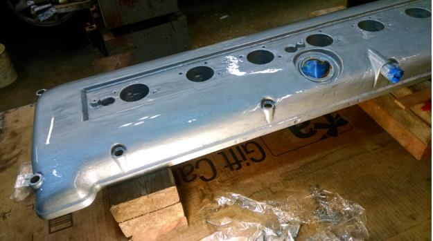
I used a model-brush to paint all of the seal-grooves. I found the paint had mended the breach in the #4 plug bore:
