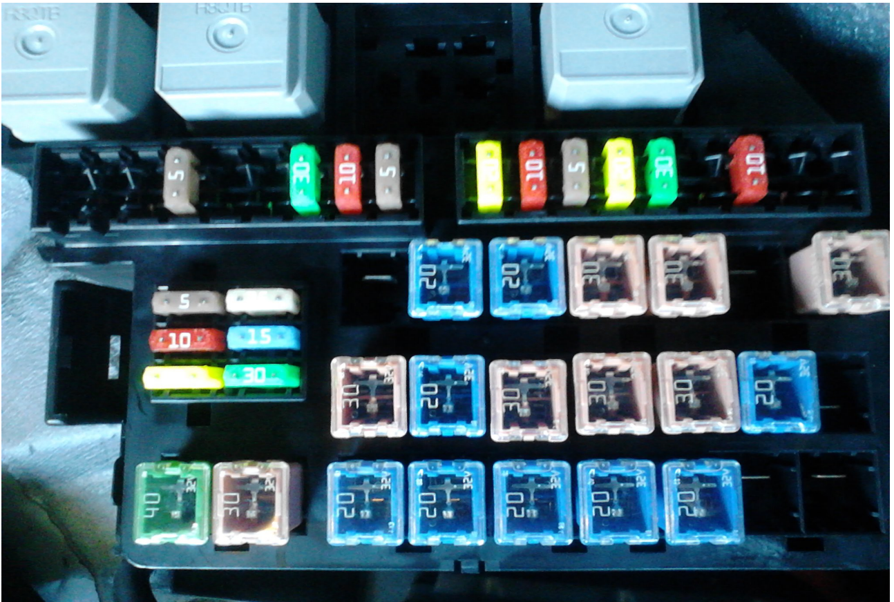
Rear Power Distribution Fuse Box in 2007 S-Type with 40A Fuse #1 at lower left corner.
