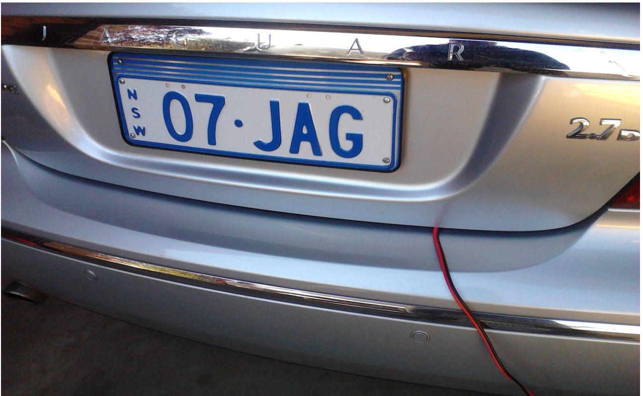
Boot/trunk lid closed to allow shut-down ... soft dust seal prevents damage to car or leads.
