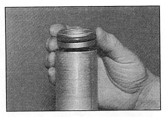
Lubricate the tube bore with a small amount of shock fluid, and insert the dividing piston (see diagram for correct orientation). With a brass rod, drive the dividing piston into the tube to a depth of 260mm (10.25") from the top of the tube (For Winston Cup shocks). Vent air pressure through the fill valve while pushing the piston into the tube or remove the valve core.
