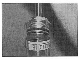
Slowly pull the piston rod, with rod guide assembly and piston head assembly, out of the shock tube.
