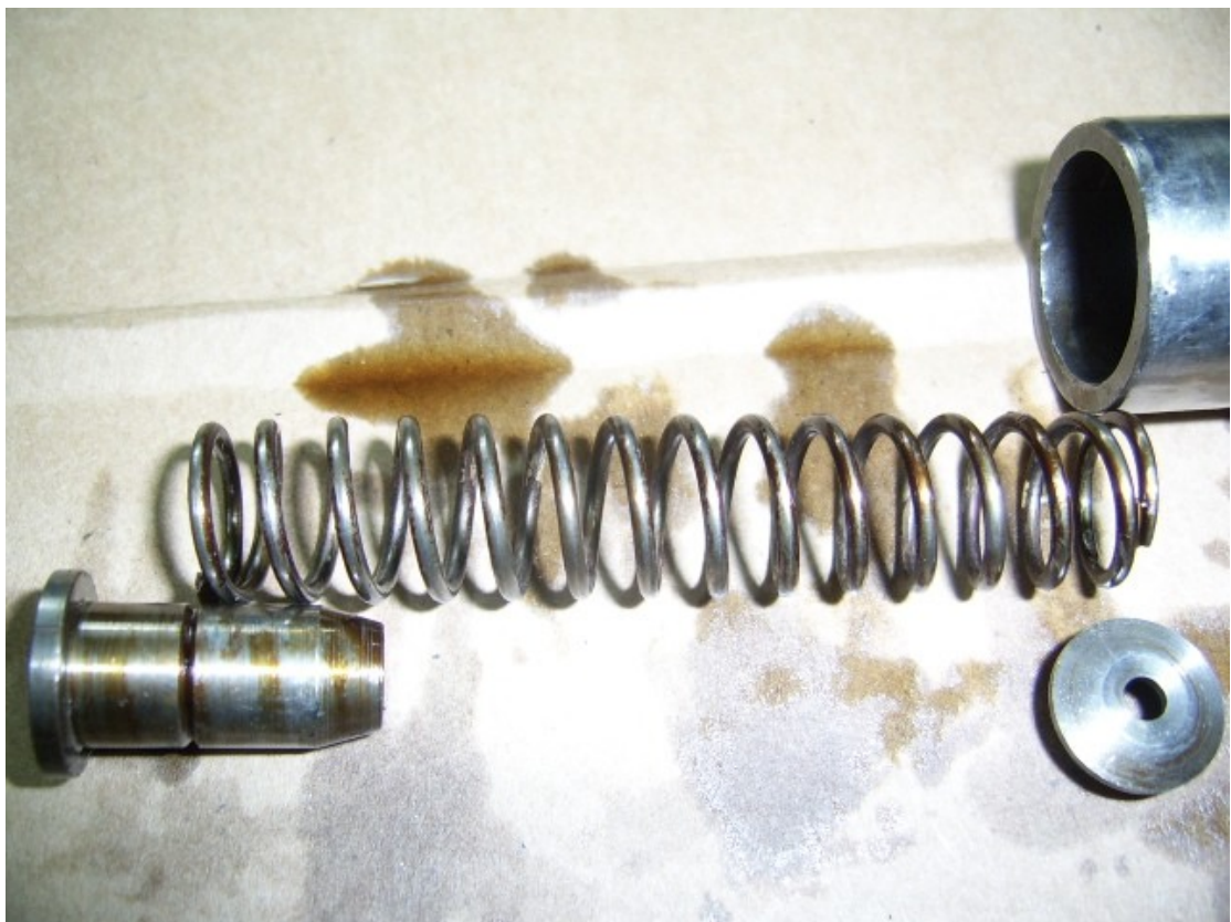
Figure 5 Showing the rivet and jet I was talking about above.
