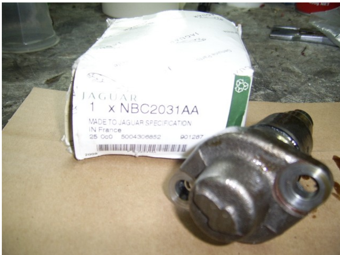
Figure 1 Tensioner as received
