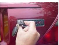
Having discovered the lock is not working you will need to press the button open the lid and remove the casing over the back side of the boot lid. This is achieved using preferably a trim removal tool, which can be purchased quite cheaply at most good Auto stores. You only need to remove the lower lip ones – 4 in total and that will give you enough access to the lock mechanism. You also need to pop the two plastic covers off the Latch cover and extract the two Torx 30 screws to remove the cover.
