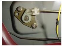
The next step involves removing the C-Clip so you can get the whole thing apart. But mark the location of the cam and note the spring fitment first.
