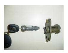
Once clean reassemble in reverse order but lubricate the moving components with a graphite grease compound as this does not absorb and attract dirt unlike traditional grease.
