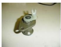
You are now going to need some way to loosen the mechanism up and soaking it in alcohol or turpentine.
