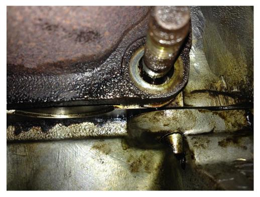
Remove Headshield, I ended up having to cut mine off as the bolts were totally knackered and rounded
