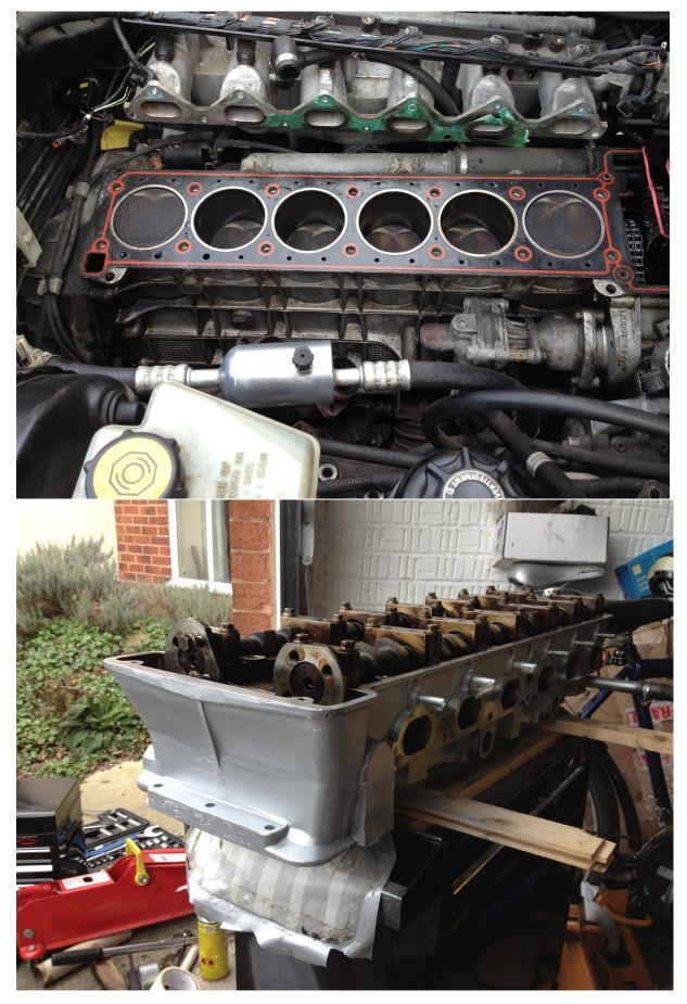
That pipe on the right of the head needs a bit of a wiggle to get out! Remember to put head on slats and NOT put flat on a surface as valves are sticking down.
