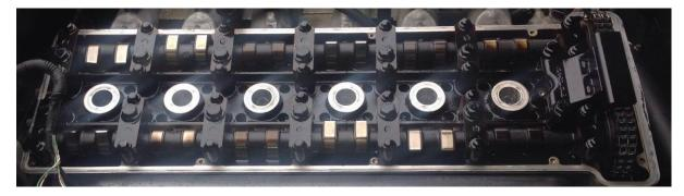
Using a 33mm spanner rotate engine to top dead centre, you will see a little "blob" in the window on the cam sensor, rotate till it is in the middle of the window. DO NOT ROTATE AGAIN
