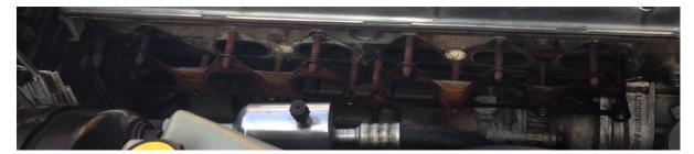
Undo all bolts holding each manifold to the head and the two on each manifold that connect the downpipe, I cleaned mine up and gave them a lick of paint
