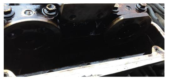
Put a laggy band (or 3) round the guides to hold the chain and everything together and out of the way
