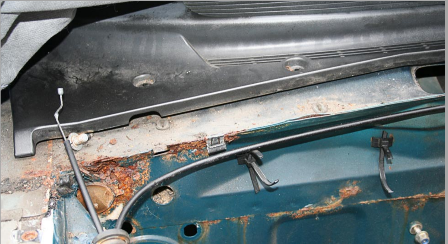
More rust. Bulkhead on both sides and the Radiator panel.
