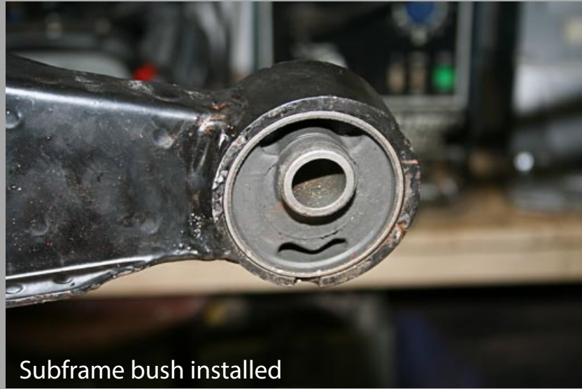
Front subframe rear bush being pressed in
