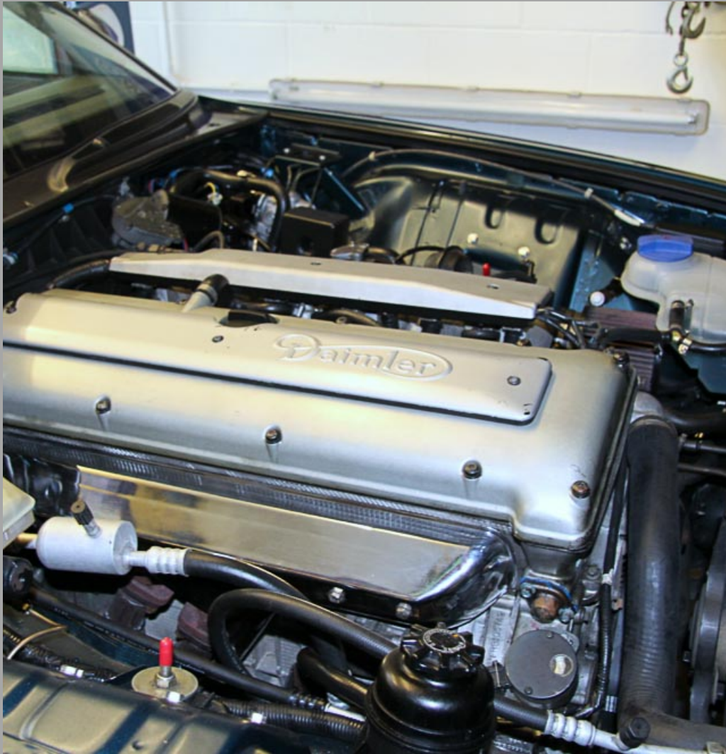
Difference in the X308 shell required some customisation under the bonnet. Note the Audi A6 header tank.
