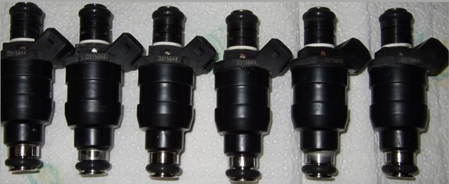
Injectors were sent off for cleaning and flow testing. A great refurbishment job by a contact from a Volvo forum.
