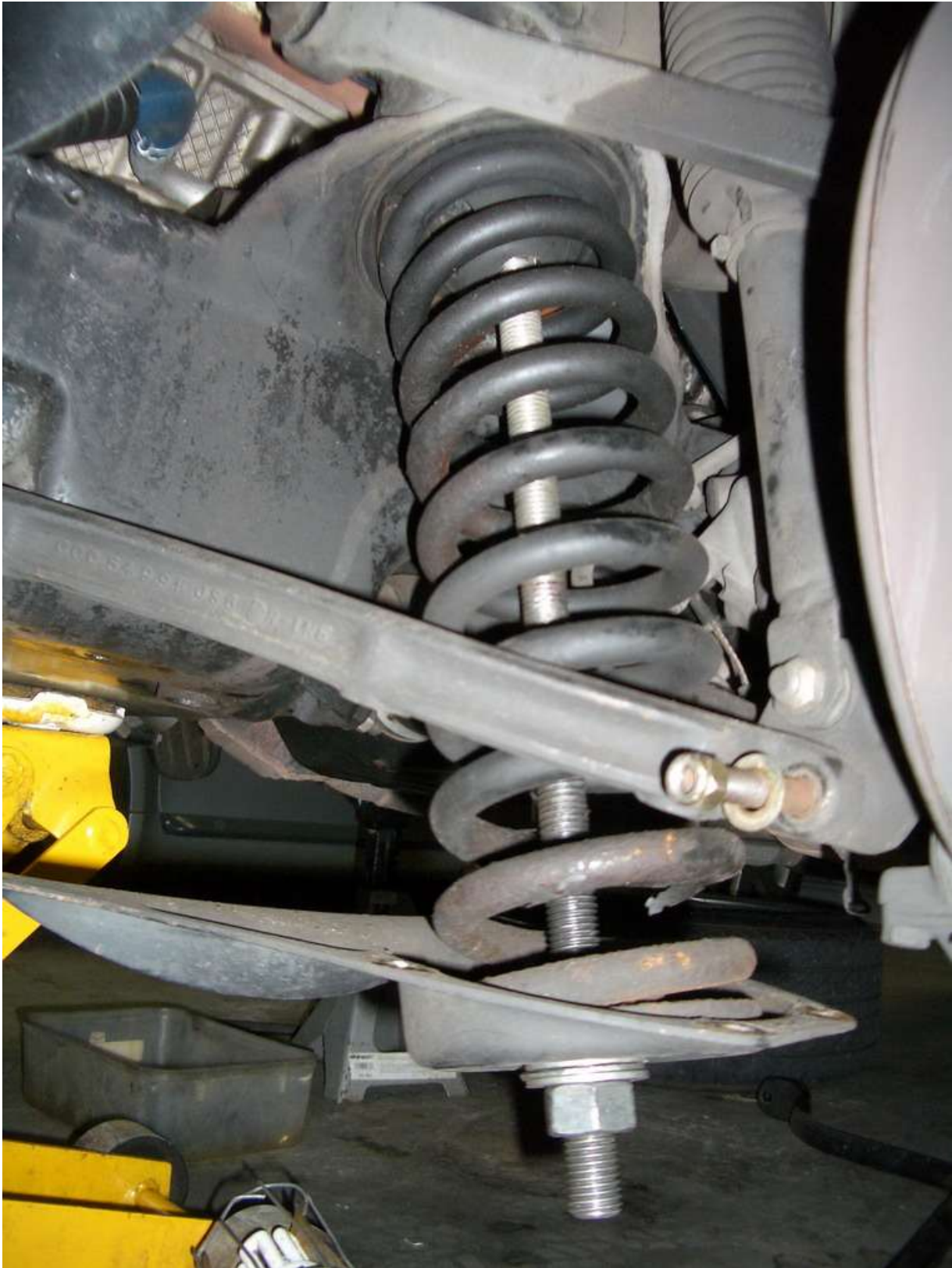
Spring compressor installed with spring at full extension.
