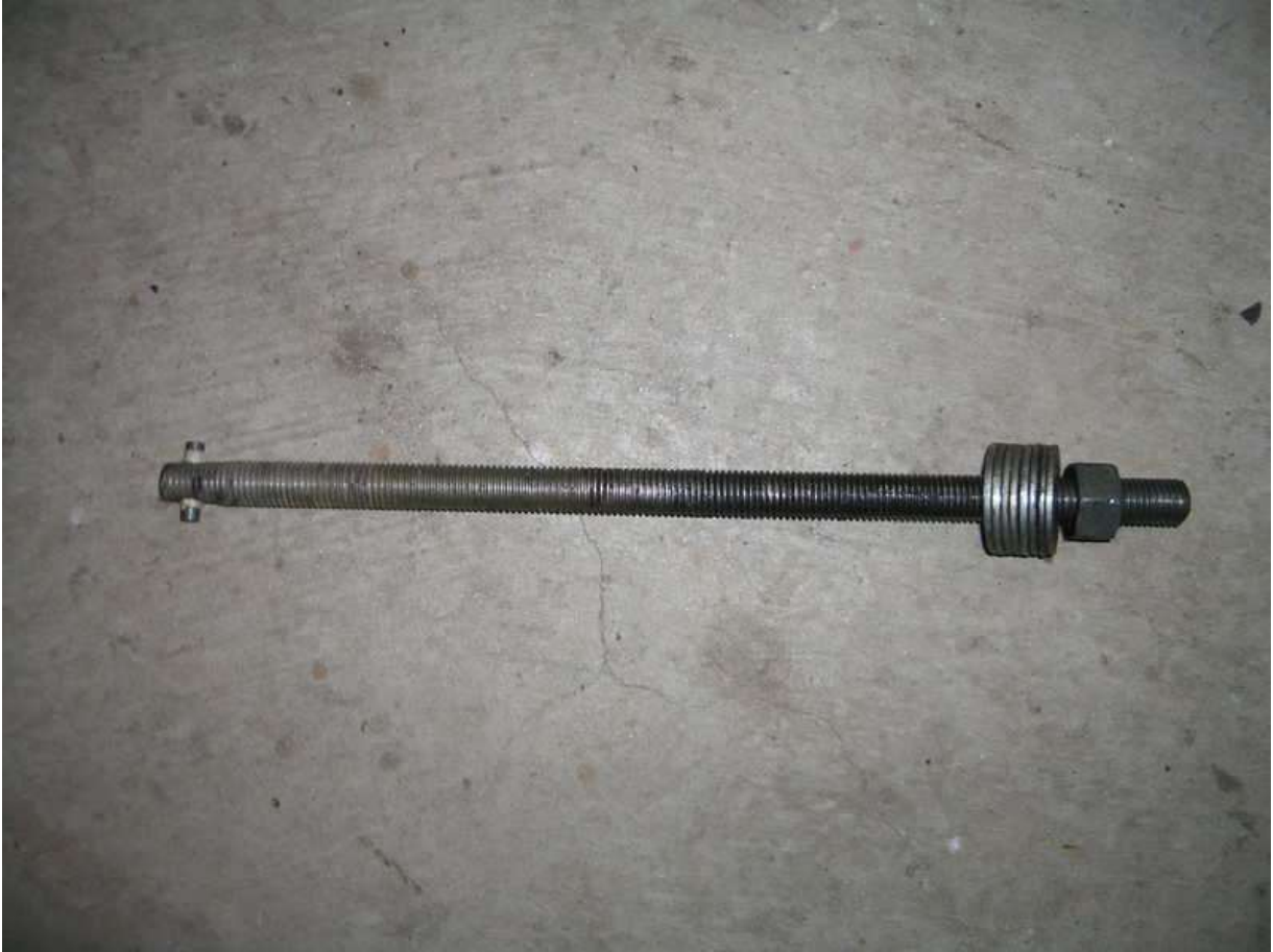
Spring Compressor as described above.
