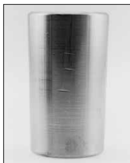
Fig. 39. Rough handling or installation damage resulted in nicks and dents in this tapered bearing roller.
