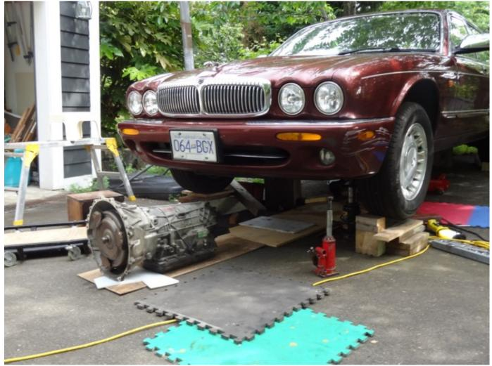
To achieve this I jacked the car up and placed the wheels on blocks to give 26" of clearance. I left the tires on as their removal would have made no difference to the job and this left me more room underneath to move around and work.
