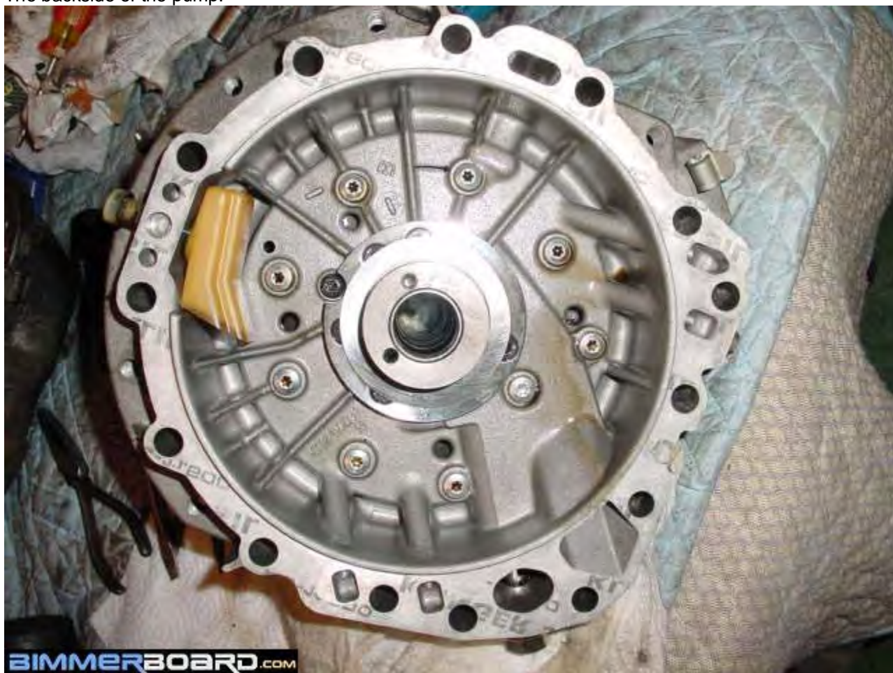
Front side of the pump. Bellhousing bolts on to this to complete the Trans rebuild.
