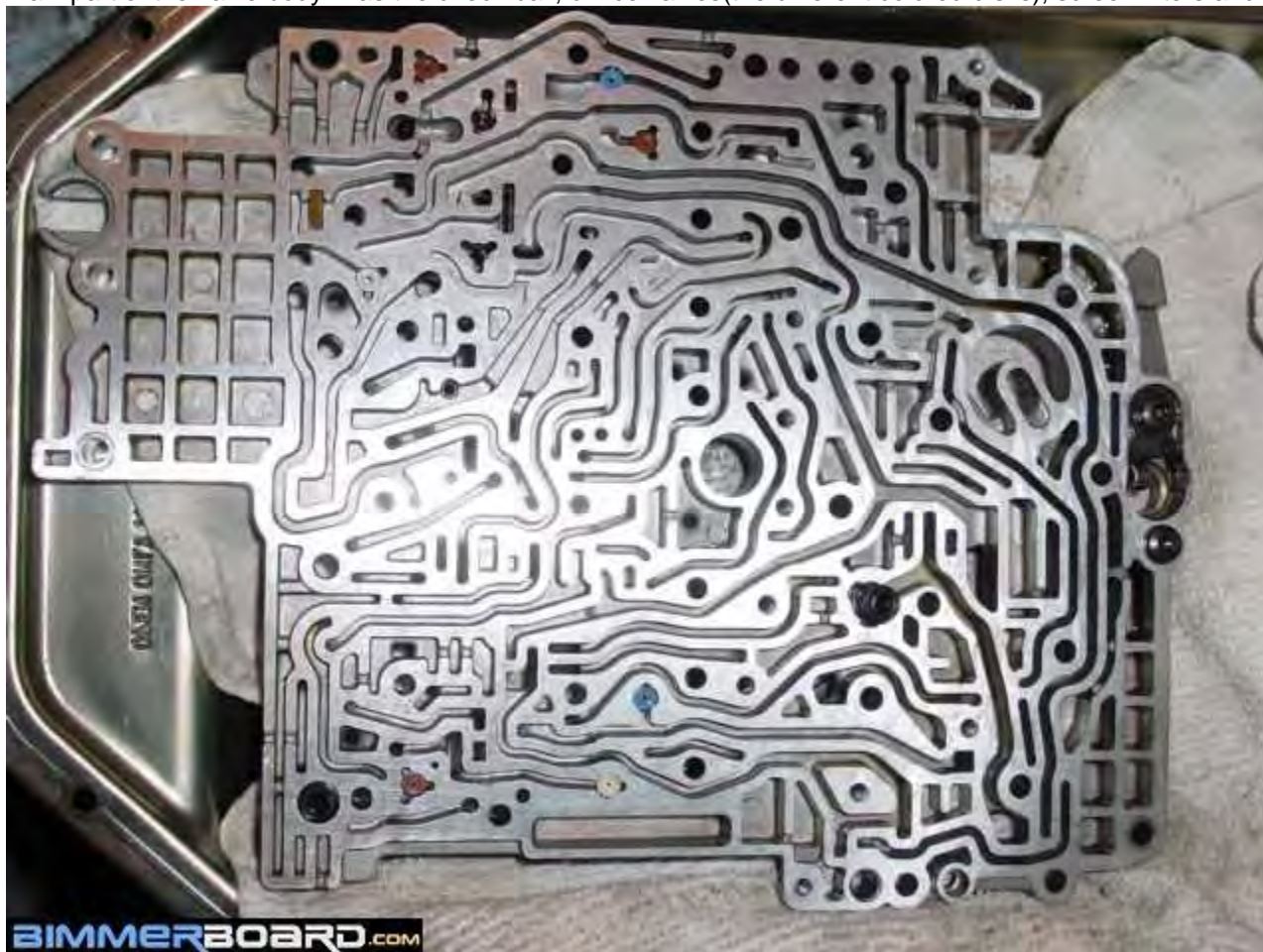
the part of the valve body you do not see when you drop the pan. The bolts go up into the trans.
