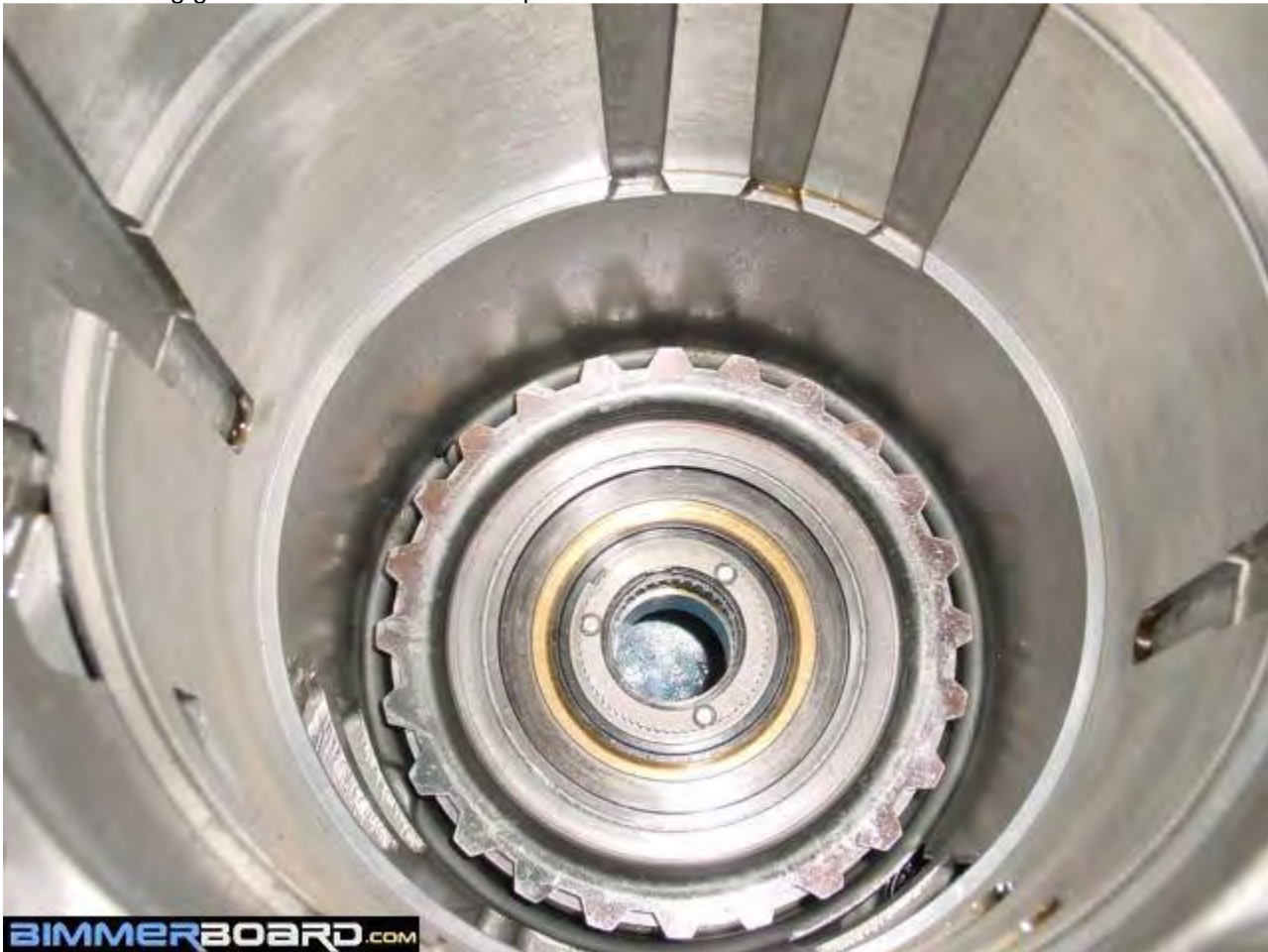
Next few photos are the parts going into the trans in the order that they went. Free wheel ring goes into the reverse clutch pack
