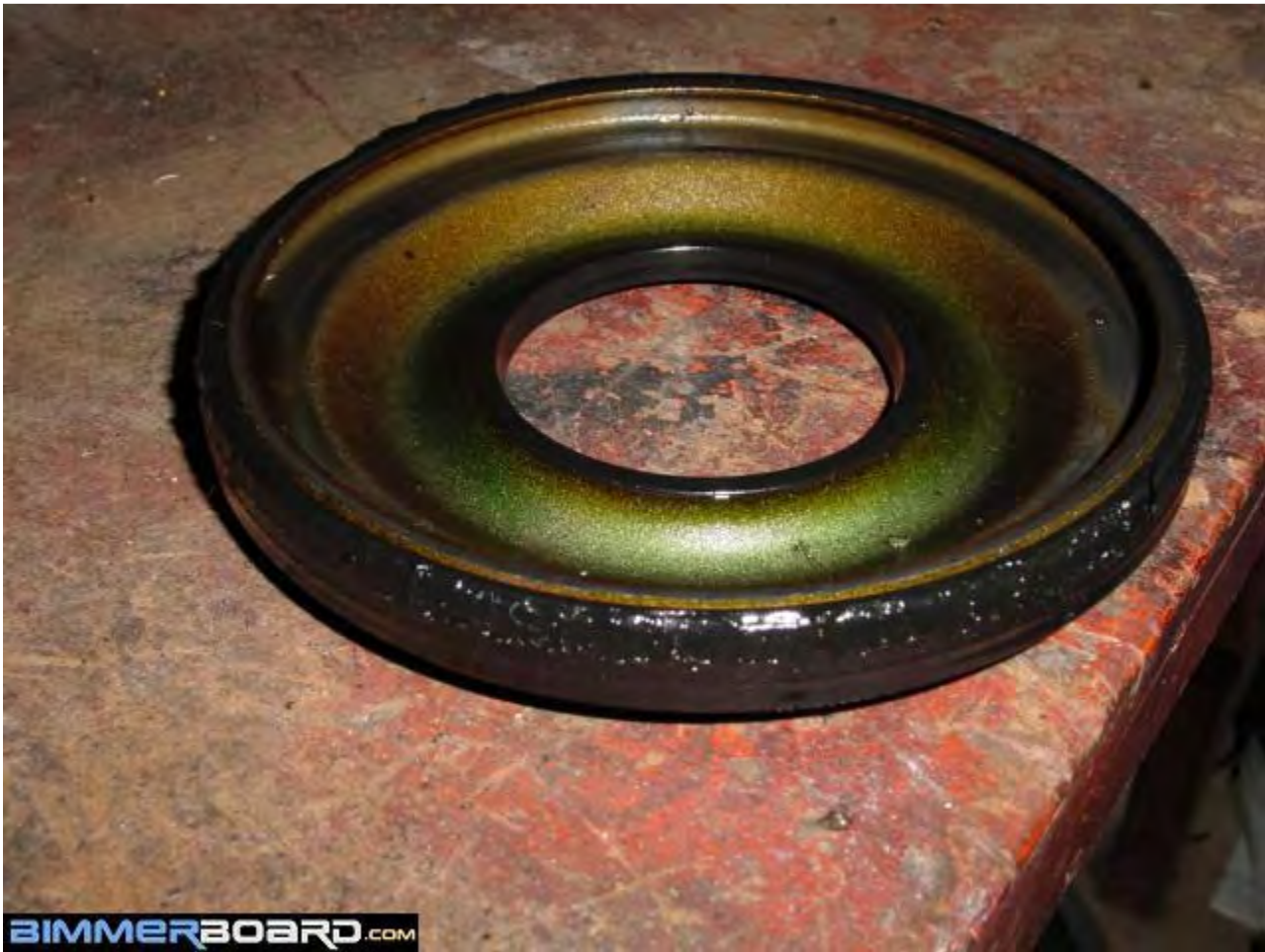
Next few photos are the parts going into the trans in the order that they went. Free wheel ring goes into the reverse clutch pack
