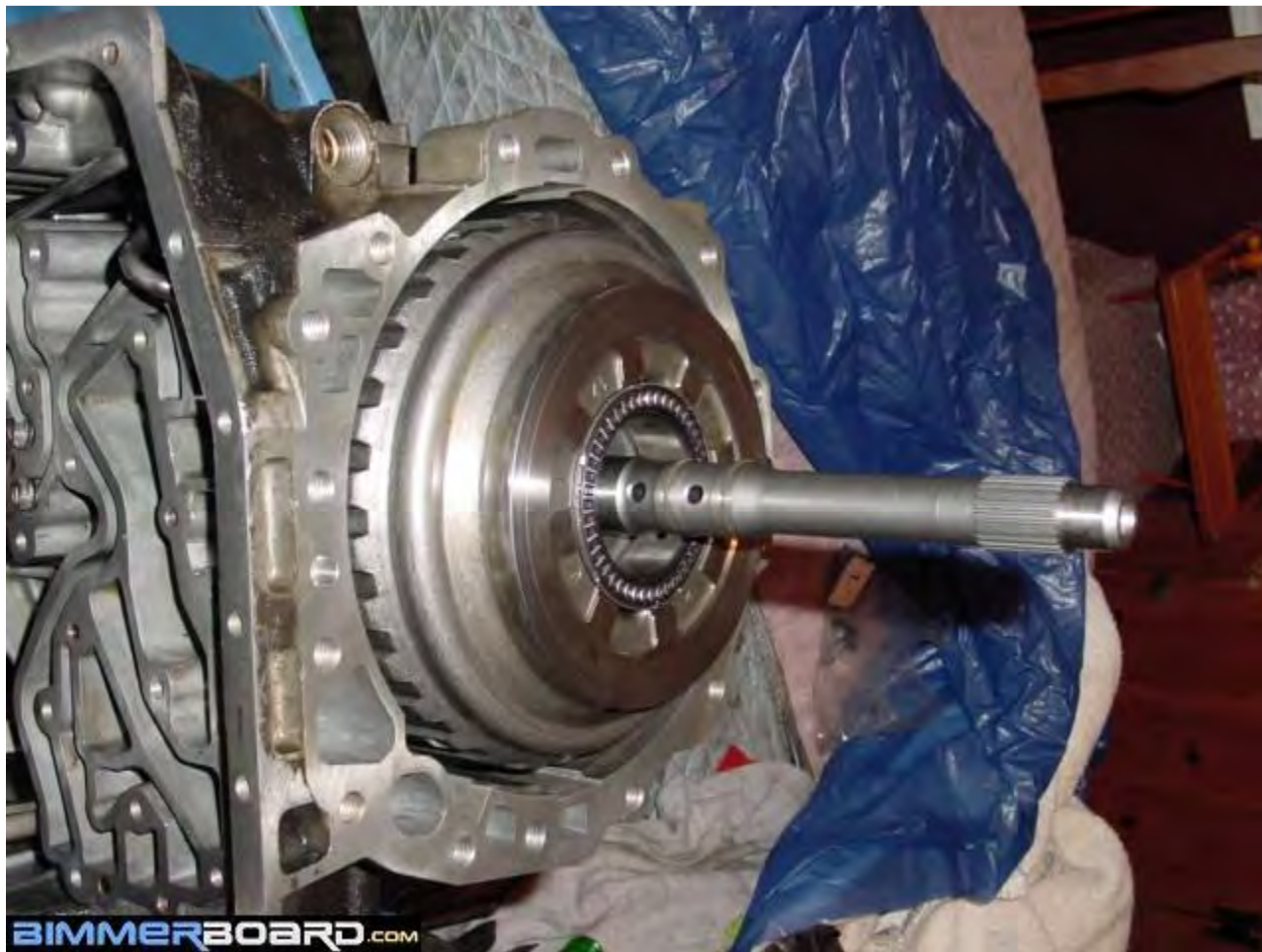
Back part of the trans. The Chevy pulley went here to pull against the spring on the reverse drum.
