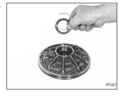
Press in sleeve 10.010/190. Assemble a new O-ring 10.014. Before putting the pump gear and pump ring gear together, lubricate them slightly with oil.
