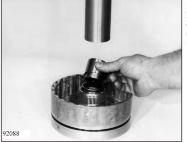
Put O-ring 75.140 on cylinder F 75.010. Press needle roller bearing 75.020 into cylinder F with press-in fixture 5x46 001 006 in the mandrel press, and secure it with snap ring 75.030.
