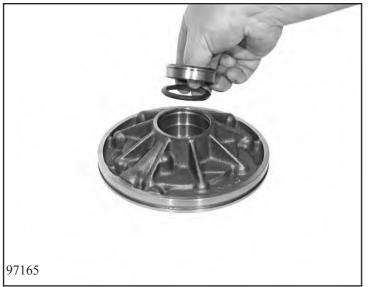
Complete pump 10.010. First put sealing ring 10.010/140 into the pump housing and press in the needle bearing 10.010/150 with assembly drift 5x46 000 954 in the mandrel press.
