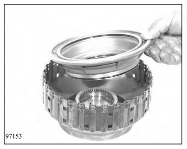
Put two O-rings (72.030, 72.040) and sealing ring 72.050 on piston B 72.010. Press piston B into cylinder B.
