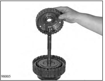
Align the discs for clutches A and B, and insert intermediate shaft 72.160, turning it as you put it in. Attach axial needle roller bearing 72.170 to the hub of inner disc car rier B using petroleum jelly. Insert inner disc carrier B 72.180, turning it as you put it in.
