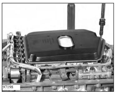
Remove the filter and the O-ring by unscrewing the 2 machine screws.
