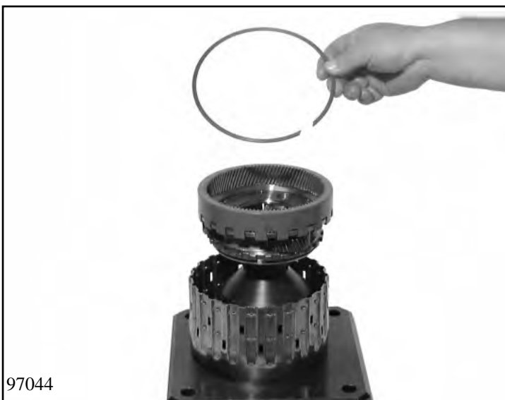
Take out the snap ring and separate planet carrier I and ring gear II from ring gear I.
