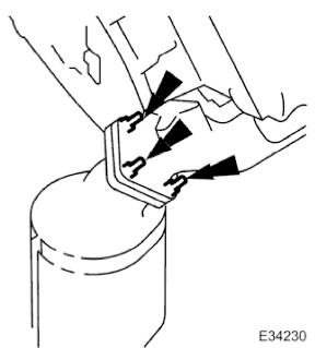
6. Remove the four nuts which secure the downpipe catalytic converter to the exhaust manifold.
