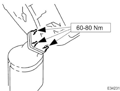
4. Tighten the nuts securing the downpipe flange to the manifold flange.
